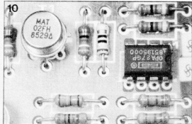
Fig. 10. The two important semiconductor devices used in the preamplifier: dual transistor MAT-02 and operational amplifier OP-27.
